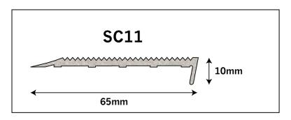
SC11 stair nosing has been extruded with a fine solid ripple trim finish to offer excellent slip resistance. Slip checked to AS 4586:2013. The SC11 is available in clear (silver) or black anodised finish for colour contrast options. It has been specifically designed to comply with the requirements of AS 1428.1-2009 and offers Class: P4 Slip Protection.
