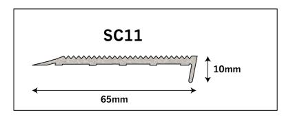
SC11 stair nosing has been extruded with a fine solid ripple trim finish to offer excellent slip resistance. Slip checked to AS 4586:2013. The SC11 is available in clear (silver) or black anodised finish for colour contrast options. It has been specifically designed to comply with the requirements of AS 1428.1-2009
