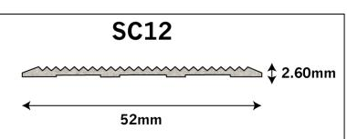
SC12 anti slip aluminium strip has been extruded with a fine solid ripple trim finish to offer excellent slip resistance. The SC12 anti slip aluminium strip is available in clear (silver) or black anodised finish for colour contrast options. It has been specifically designed to comply with the requirements of AS 1428.1-2009 and offers Class: P5 slip protection.
