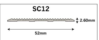
SC12 anti slip aluminium strip has been extruded with a fine solid ripple trim finish to offer excellent slip resistance. The SC12 anti slip aluminium strip is available in clear (silver) or black anodised finish for colour contrast options. It has been specifically designed to comply with the requirements of AS 1428.1-2009
