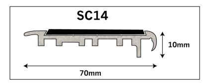
SC14 carpet tile nosing for use on carpet tiles, direct stick carpets or vinyl. Specially designed for situations that need to comply with the requirements for stair nose not to extend down the riser more than 10mm, as specified in AS 1428.1-2009. All Staircare inserts have been slip checked to AS 4586:2013.
