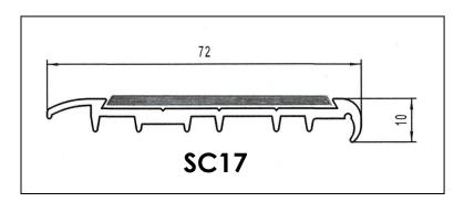
SC17 carpet stair nosing has been designed for use on thick carpet or carpet with underlay. Designed for situations that need to comply with the requirements for stair nose not to extend down the riser more than 10mm, as specified in AS 1428.1-2009. All Staircare inserts have been slip checked to AS 4586:2013.
