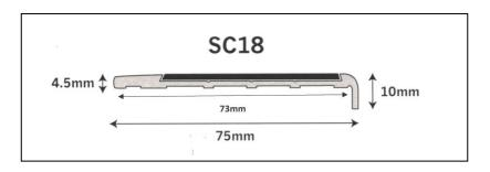
SC18 recessed stair nosing can be recessed into new or existing floor finishes; including concrete, tiles, timber, carpet or vinyl. The stair nosing can be fitted with different styles of insert to suit internal or external applications. All Staircare inserts have been slip checked to AS 4586:2013. SC18 fully complies with the requirements of AS 1428.1-2009
