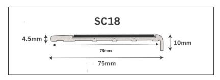
SC18 recessed stair nosing can be recessed into new or existing floor finishes; including concrete, tiles, timber, carpet or vinyl. The stair nosing can be fitted with different styles of insert to suit internal or external applications. All Staircare inserts have been slip checked to AS 4586:2013. SC18 fully complies with the requirements of AS 1428.1-2009
