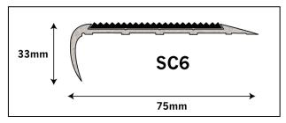
SC6 Stair Nosing has been designed for both carpeted and hard surface stairs. The aluminium base is anodised or powder coated. SC6 can be fitted with three different types of anti slip insert. All Staircare inserts have been slip checked to AS 4586:2013.
