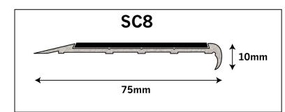
SC8 stair nosing has been designed for use on hard surface stairs, either indoor or outdoor. The nosing can be fitted with four different styles of insert to suit various applications. All Staircare inserts have been slip checked to AS 4586:2013. SC8 fully complies with the requirements of AS 1428.1-2009
