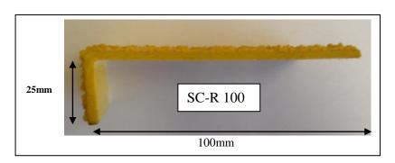
Staircare SC-R 100 have been designed to offer lasting slip resistance. They are made from a composite material that is suitable for use in harsh environments; including, high exposure to salt water. During the manufacture process silicon carbide is incorporated to form an inseparable gritted surface. SC-R 100 are available in yellow with UV protection and a heavy duty silicon carbide anti slip grit for serious slip protection.
