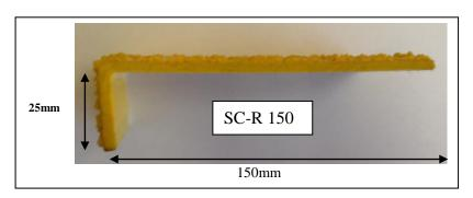
Staircare SC-R 150 have been designed to offer lasting slip resistance. They are made from a composite material that is suitable for use in harsh environments; including, high exposure to salt water. During the manufacture process silicon carbide is incorporated to form an inseparable gritted surface. SC-R 150 are available in yellow with UV protection and a heavy duty silicon carbide anti slip grit for serious slip protection.
