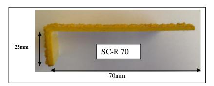
Staircare SC-R 70 have been designed to offer lasting slip resistance. They are made from a composite material that is suitable for use in harsh environments; including, high exposure to salt water. During the manufacture process silicon carbide is incorporated to form an inseparable gritted surface. SC-R 70 are available in yellow with UV protection and a heavy duty silicon carbide anti slip grit for serious slip protection.
