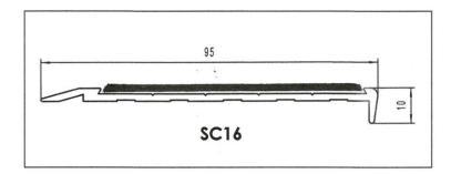
SC16 stair nosing is a solid tread suitable for repair of broken step edges or to offer effective protection of stairs with heavy foot traffic. It is available with a 74mm wide SC-R solid carborundum or carborundum anti slip tape insert. SC16 fully comply with AS 1428.1-2009. All Staircare inserts have been slip checked to AS4586:2013.
